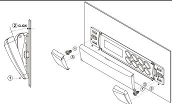
7.4 XW10L: MOUNTING WITH KEYBOARD COVER OPENING UPWARD
